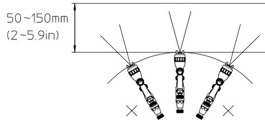
Pulling the trigger of the gun with the pattern adj. Set and fully opened adjust the air regulator in the spray booth to obtain 0.5~1.0 bar ( 7~14 PSI) at the gun inlet as issued on specifications table ahead. In this way the gun will atomize within 0.7 bar (10 PSI) inside air cap.
